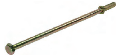
84-82107 Thru Bolt Hex Head w/Split Lock Washer Dim. : M6 x 1.0 x 150mm L For: Denso OSGR waffle 1.4kw Starter Note: Field Case to DE and DE to CE
