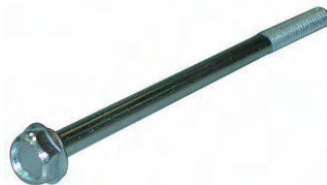
84-82169 Thru Bolt Hex Washer Head Dim. : M6 x 1.0 x 95mm L 100.7mm OAL 23mm Threaded L For Mitsuba PMGR Starter Lester: 17958
