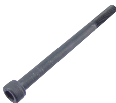
84-82179 Thru Bolt Socket Head Dim. : M6 x 1.0 x 84.5mm L Note: DE to Solenoid
